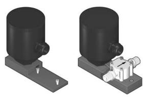
This Kit consists of an additional IP65 housing mounted aside the sensor via a PVC plate. It is a blind transmitter designed to convert the signal from the sensor into a 4-20 mA output for long distance transmission.
