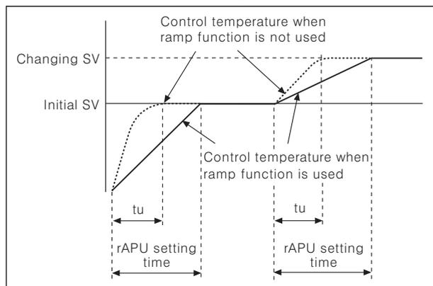
It makes delay rising temperature when change the set value at stable control status or delay the initial rising temperature as like above picture.
