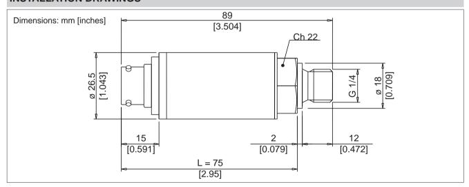
**Dimensions:** TPSADA, due to the autozero & span board, is 5 mm (0.197 in) longer, so dimension "L" on TK data sheet
