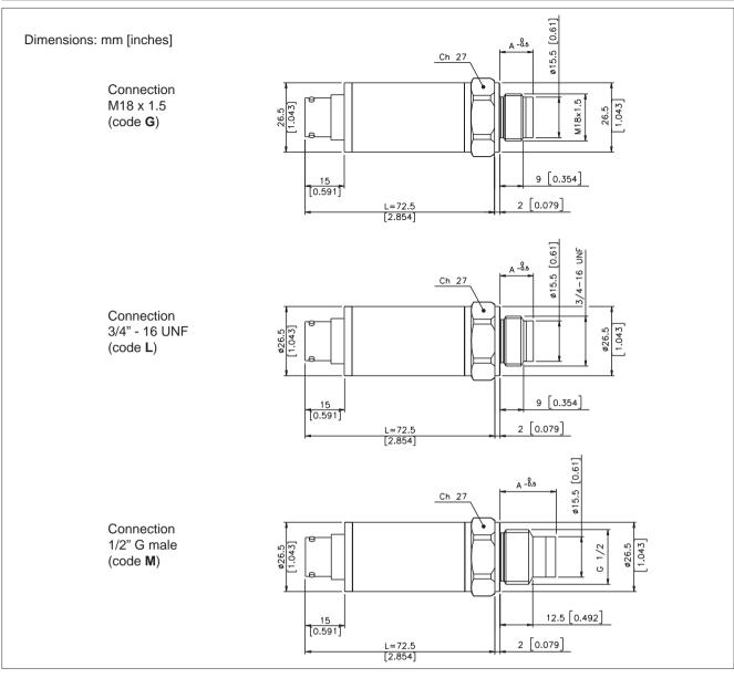
ATTENTION: for installation use a maximum torque force of 40Nm
