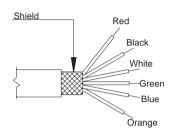
Shielded cable 6x0.25 - 1m Protection IP65
