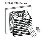
\*Mount the product on the panel and securely push the bracket in using a tool, as shown in the diagram.
