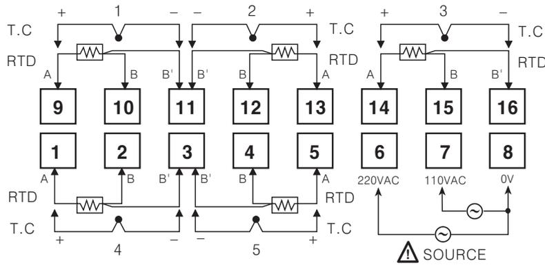
※RTD(Resistance Temperature Detector) : Pt 100Ω (3-wire type) ※Thermocouple : K, J
