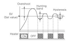
As like above picture, the control value is up and down by set value, it is called Hunting. And Overshoot is occurred at initial point when just nower on
