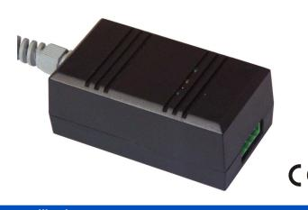
The SRS-2/4-Z45 converter module is used to connect MASTER devices with an RS 232 port to an RS 485 bus. The module supports devices, which control Tx switching using the RTS signal and devices, which do not control Tx switching using the RTS signal (Tx switching is then fully automatic). For example, a suitably programmed PC computer can function as the system MASTER device.
