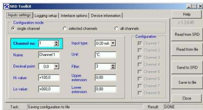
The **SRD Toolkit** software enables configuration reading and writing operations, updating the device firmware and obtaining basic information on SRD-99-type devices through RS-485 serial interface. This application enables to quickly and easily define device parameters in one of three possible configuration models. The set of parameters can be transmitted directly to the device or stored in a file for future use.
