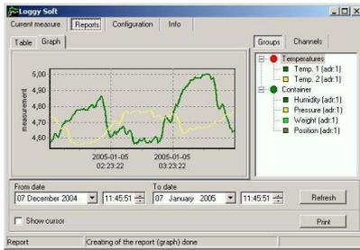
The **Loggy Soft** program enables the visualization, archiving and printing of measurements (e.g. temperature, humidity, pressure) stored in SRD-99-type device memory. Work with SRD-99-type devices takes place through an RS-485 serial interface. Connecting a network of units to a serial port (RS-232) or USB port of a PC is possible thanks to a converter (RS-485 to RS-232 or RS-485 to USB) produced by SIMEX.
