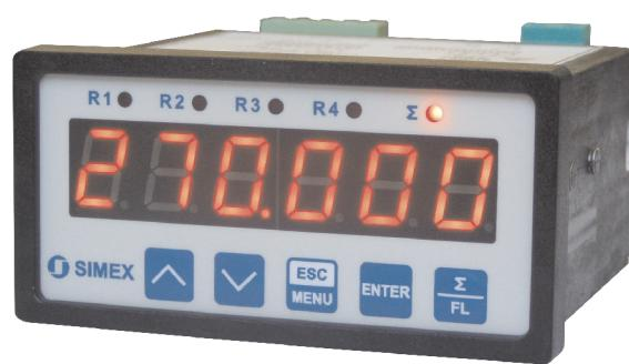
**SPP-94** are the flow meters designed to work in tandem with the pulse flow transducers with current input of 0-20 mA or 4-20 mA. Wide balance range (up to 13 significant digits) enables flow volume control for a long time. The counters have 2 or 4 relay or OC outputs, depending on the actual instantaneous value of the flow or balance (only R1 output).
