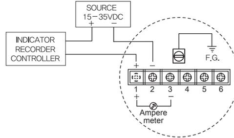
※ You can check 4-20 mA output by connecting an ampere meter. (impedance: max. 30 Ω)
