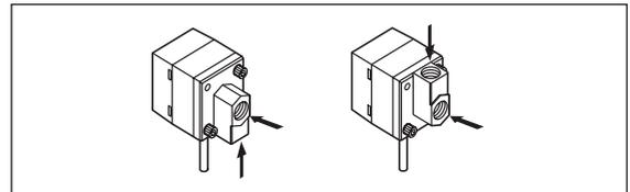
3. Please use seal tape at port plug in order to prevent pressure leak.
