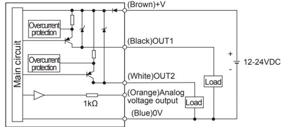
※There is no short-circuit protection in analog voltage output. Do not connect this output to power supply or capacitive load directly.
