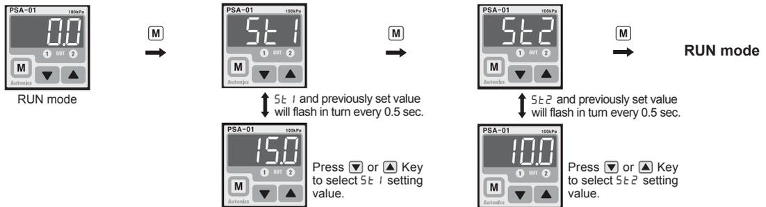
※5.1 setting range : Min. display pressure < 5.1 ≤ Max. display pressure
