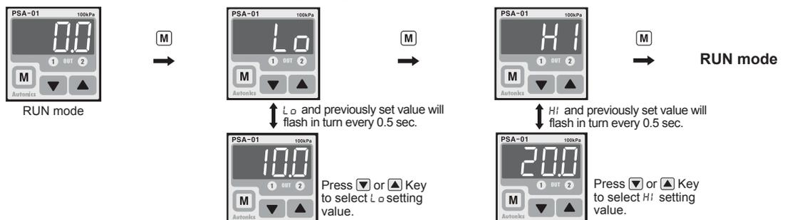
※Low value setting range : Min. display pressure < Lo ≤ Max. display pressure
