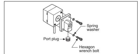
5. Please connect it by using spanner(13mm) at the metal part in order not to overload on the body when connecting one touch fitting.
