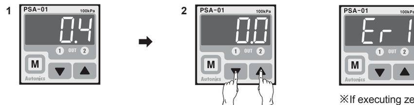
1. In state of atmospheric pressure during RUN mode, press  $\nabla$  key and  $\blacktriangle$  key at the same time for over 1sec.
