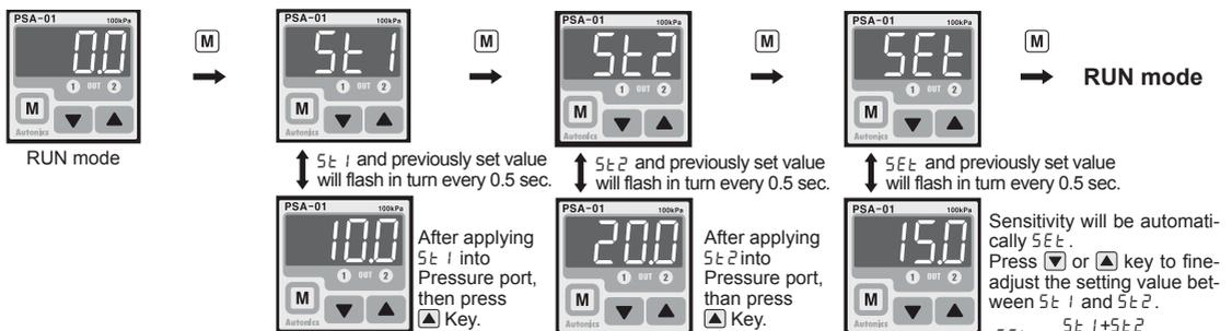
※5.1 setting range : Min. display pressure < 5.1 ≤ Max. display pressure – 1% of rated pressure
