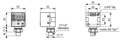
$\times$ (A) PT1/8" model(Standard): 8, NPT1/8" model: 8, 7/16"-20 UNF model: 11  $\times$ 1: Only for PT1/8" model, NPT1/8" model
