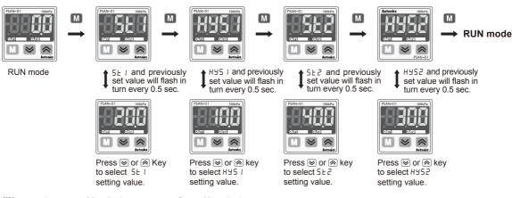
※5₺ / setting range : Min. display pressure < 5₺ / ≤ Max. display pressure</p>
