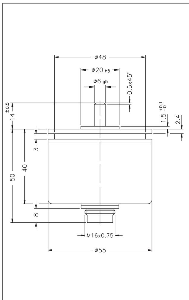
**Important:** all the data reported in the catalogue linearity, lifetime, temperature coefficient are valid for a sensor utilization as a ratiometric device with a max current across the cursor  $I_c \leq 0.1 \mu\text{A}$ .
