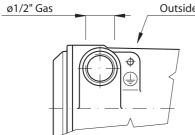
Die-cast aluminium casing UNI5076
