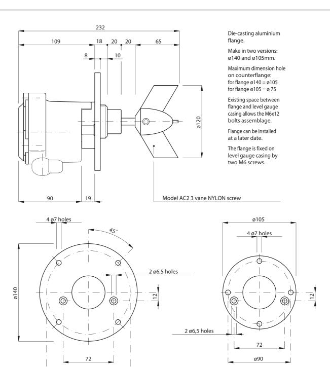
Level gauge can be delivered with extension, with or without protection, the length is defined by the buyer during the order.
