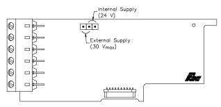
For Quad Sourcing Plug-in Card (PAXCDS40), set the jumper for internal or external supply operation before applying power.
