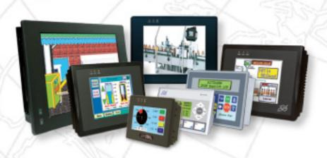
The configuration software includes recipes, menus, alarms, and the ability to create over 500 screens. Designed for harsh industrial environments, this OIT carries a Class I Division 2 rating and operate under a wide temperature range.
