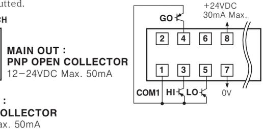
●MT4W-□□-48/ MT4W-□□-49 (Triple NPN/PNP open collector output+RS485 output)
