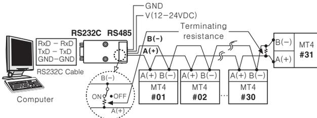
※Autonics SCM-38I is recommended to use for RS232C to RS485 converter.
