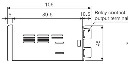
※ There is no Relay contact output terminal block in indication type.
