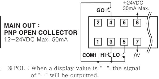
●MT4W-□□-44/ MT4W-□□-45 (Triple NPN/PNP open collector output+Current output)
