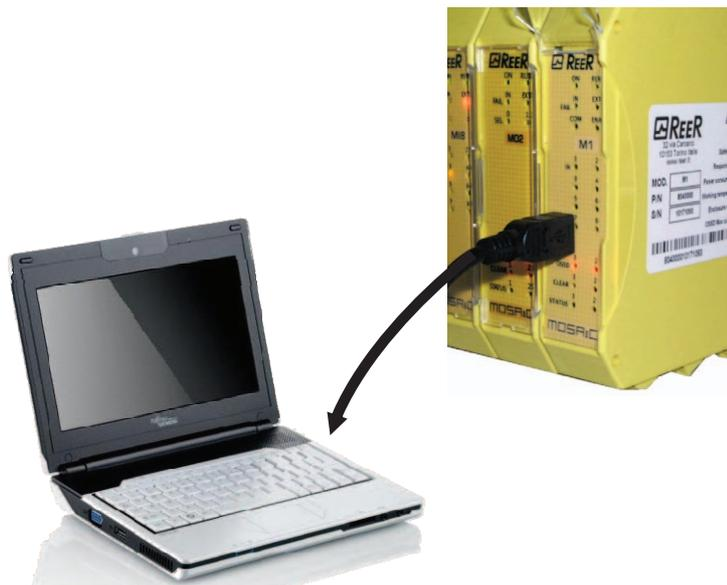
Figura 2 - Conector delantero USB 2.0
