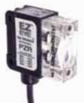
Type V8 Convergent .5" "V" Axis Narrow beam optics that focus at a sensing range of .5". Useful for sensing small parts. Also useful for proximity sensing (range of .25" to 5") to minimize response to reflected light from background objects.
