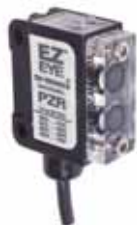
Type O4 Proximity Wide beam optics useful for short-range sensing of transparent, translucent or irregular shaped shiny objects.
