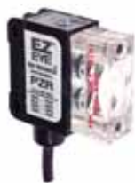
Type V4A Convergent Aperture 1" "V" Axis Aperture provides spot focus light beam at a sensing range of 1". Useful for sensing small parts or narrow gaps. Also useful for proximity sensing (range of 1" to 5") to minimize re- sponse to reflected light from background objects.
