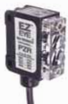
Type V6 Convergent 1.5" "V" Axis Narrow beam optics that focus at a sensing range of 1.5". Useful for sensing small parts. Also useful for proximity sensing (range of 1.5" to 8") to minimize response to reflected light from background objects.
