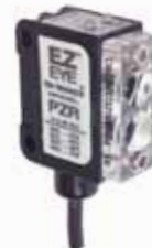
Type R5 Polarized Anti-Glare Retroreflective Polarized to reduce response to "hot spot" glare from shiny surface of detected object. Use with red light source.
