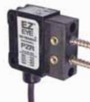
Type F4 Glass Fiberoptics Adapts for use with a wide variety of glass fiberoptic light guides (.187 O.D.) for both the proximity and opposed sensing modes.
