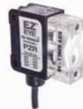
Type V4 Convergent 1" "V" Axis Narrow beam optics that focus at a sensing range of 1". Useful for sensing small parts. Also useful for proximity sensing (range of 1" to 5") to minimize re- sponse to reflected light from background objects.
