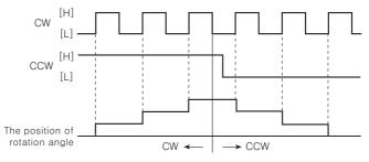
Note) When using the 2-PULSE input method, do not input CW and CCW at the same time.
