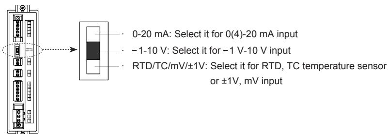
This unit is multi input product. Select the proper input with the input type selection switch and select this input type in *I n - P* in program mode. The setting of input type selection switch and the input type *I n - P* parameter should be same and it can display the proper measurement value. Factory default is 0-20 mA.
