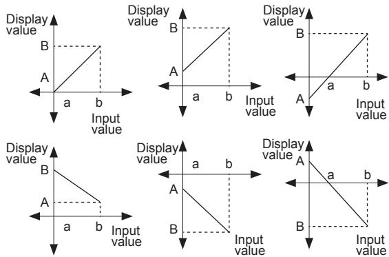
Display scale function is able to change display value for max./min. measured input by setting high limit scale [ H-SC ] and low limit scale [ L-SC ] in program mode.
