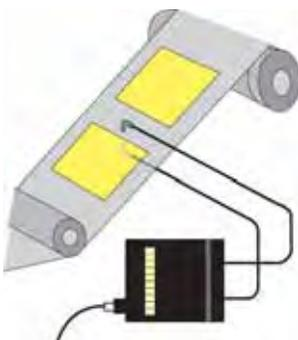
Best method to detect self-adhesive labels on backing material.
