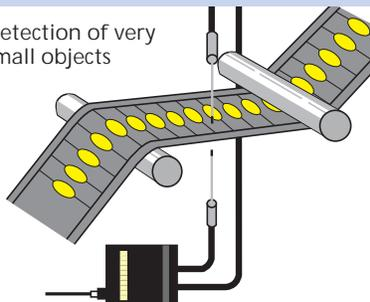
Polarized light detection of plastic containers
