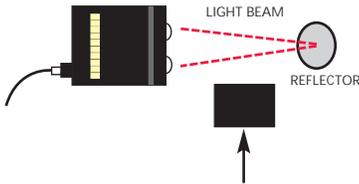
Retroreflective mode. Use with reflector to detect medium to large size opaque objects.
