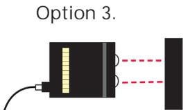
Proximity (divergent beam) mode sensing is useful in detecting some large size translucent/transparent objects from longer range. Generally speaking, there must be substantial gaps between objects for this mode to be effective.
