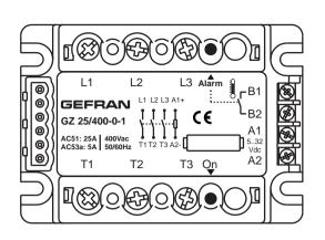
L1: Phase 1 input L2: Phase 2 input L3: Phase 3 input T1: Phase 1 output T2: Phase 2 output T3: Phase 3 output A1: Control signal (+) A2: Control signal (-) B1: Alarm output (+) option
