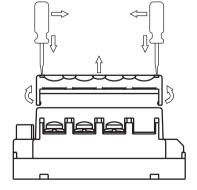
Insert the screwdriver to facilitate opening of the cover
