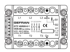
L1: Phase 1 input L2: Phase 2 input L3: Phase 3 input
