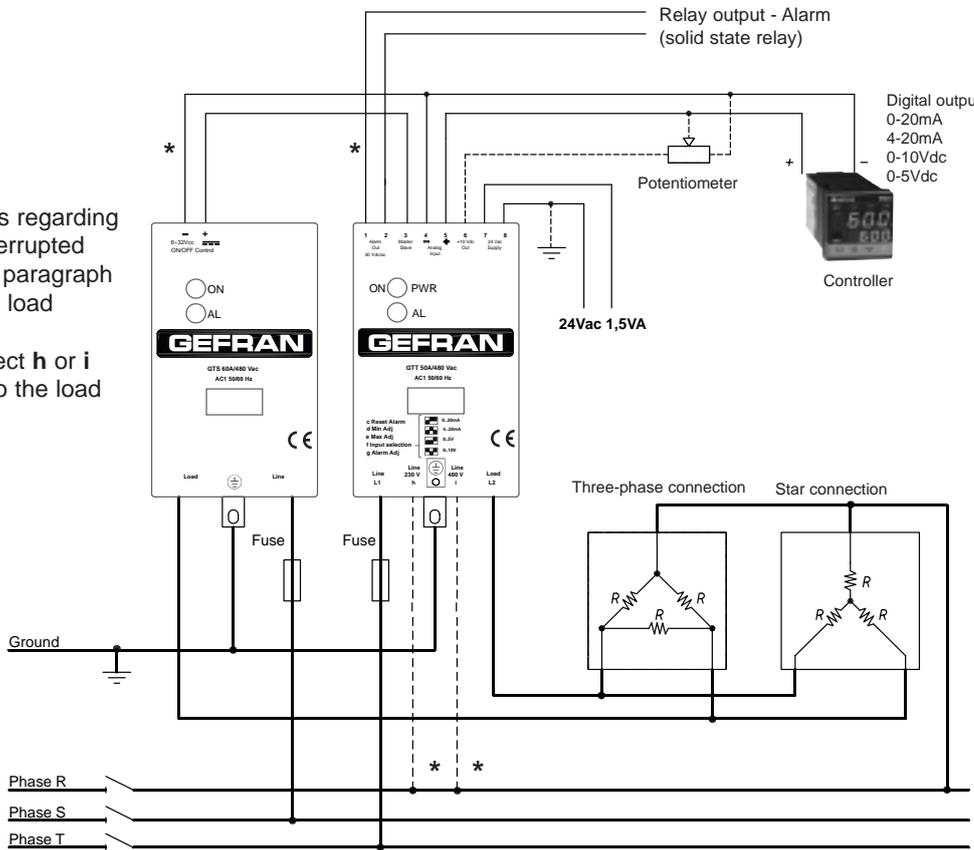
Three-phase star connection with neutral using one GTT in Master configuration and two GTSs in Slave configuration.
