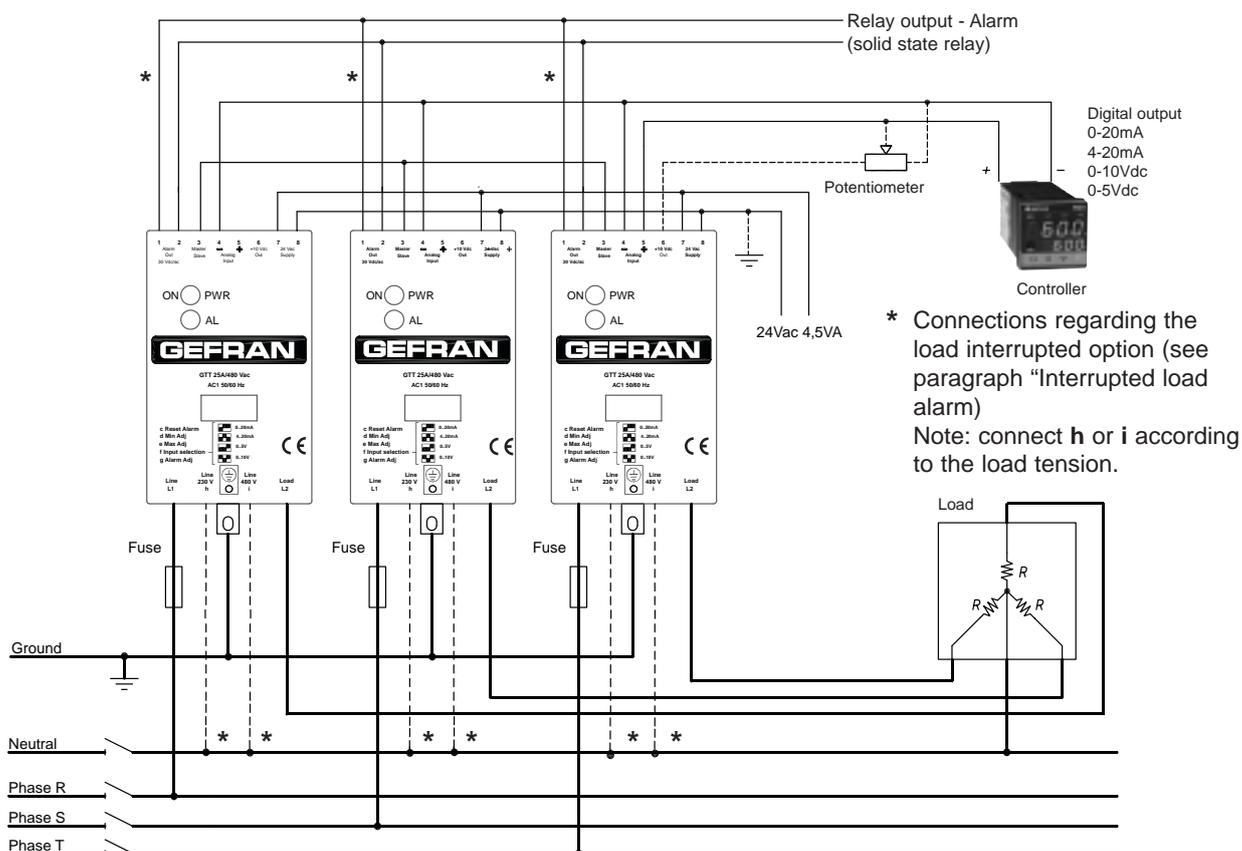
Star or delta three-phase connection without neutral, with control of three phases.
