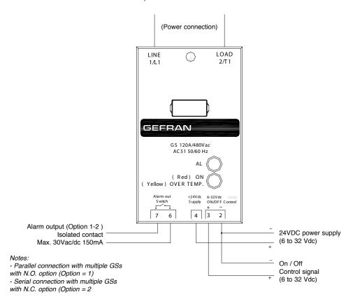
Connection example for GS with VDC control with PNP alarm output option (only Models GS-xx/xx-D-3 or GS-xx/xx-D-4)
