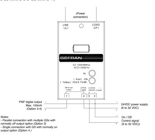
Connection example for GS with VDC control with alarm output option (Option 1) (only Models GS-xx/xx-A-1) (Power connection) LOAD 1/L1 **GEFRAN** GS 120A/480Vac AC 51 50/60 Hz (Red) ON ( Yellow) OVER TEMP. 20-260Vac/dc ON/OFF Control Alarm out 3 2 7 6 On / Off Alarm Output VAC control signal Isolated contact (20 to 260 VAC) Max. 30VAC/DC 150mA Notes:
