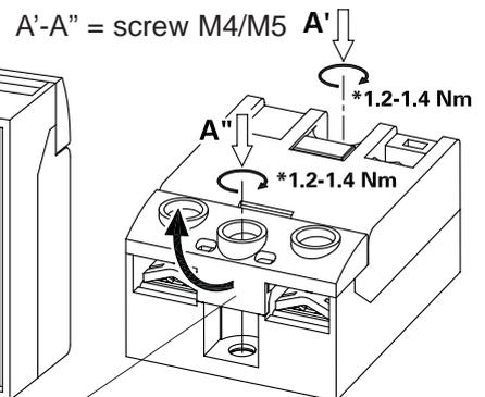
Raise the guard to access the fastening hole or the terminals
