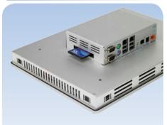
The use of Compact Flash type mass storage and/or DiskOnModule with their easy removal/replacement, is an intrinsic safety of high reliability and robustness.
