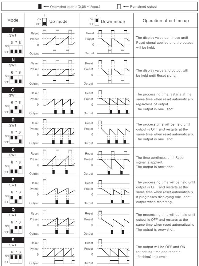
※ Time Up: When processing time reaches to setting time.
