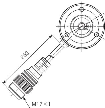
※ Connector cable is customizable and see M-46 for specifications.
