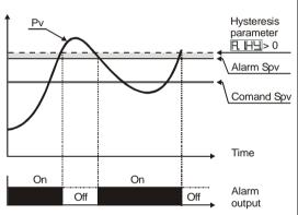
Lower deviation alarm value of alarm setpoint less than "0" and hysteresis value greater than "0" (Par.28 R HH) > 0).
