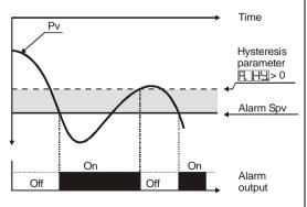
Absolute alarm with controller in cooling functioning (Par.11 FLE) selected EDDL) and hysteresis value greater than "0" (Par.28 FL HH) > 0).
