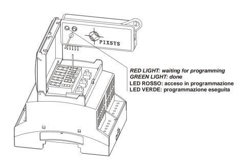
With the controller not connected to power supply.
