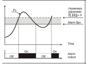
Absolute alarm with controller in heating functioning (Par.11 Fighther) selected Fighther and hysteresis value less than "0" (Par.28 Fighther) < 0).
