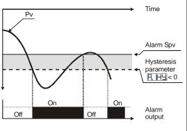
Absolute alarm with controller in cooling functioning (Par.11 同正上 selected □□□L) and hysteresis value less than "0" (Par.28 日 田里 < 0).
