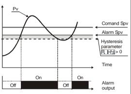
Upper deviation alarm <u>value of alarm setpoint less than "0"</u> and <u>hysteresis value greater than "0"</u> (Par.28 []. []] > 0).
