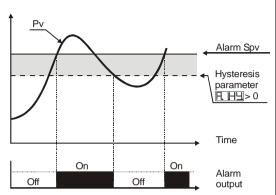
Absolute alarm with controller in heating functioning (Par.11 HELL selected HERL) and hysteresis value greater than "0" (Par.28 R HH) > 0).
