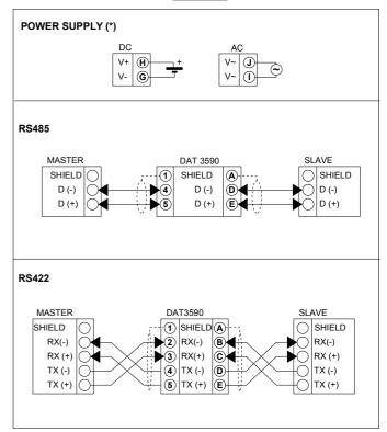
(\*) Note: for UL installation the device must be powered using a power supply unit classified NEC class 2 or SELV
