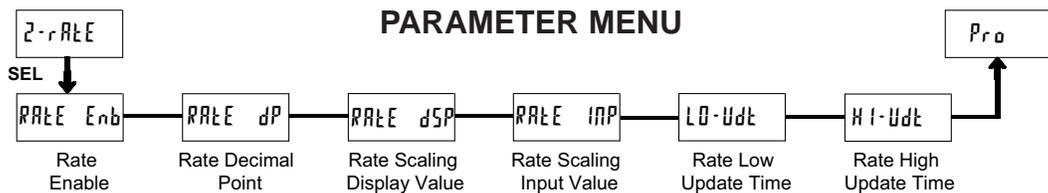
Module 2 is the programming for the rate parameters. For maximum input frequency, Rate Enable should be set to NO when not in use. When set to NO, the remaining rate parameters are not accessible. The rate value is shown with an annunciator of "R" in the Display Mode.
