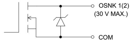
Note: Output Common is not isolated from DC Power Common. Load must be wired between OSNK terminal and V+ of the load supply.
