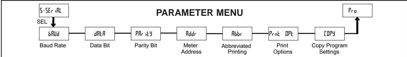
The Serial Setup Parameters are only active when one of the optional serial communication/programming cards is installed in the meter.
