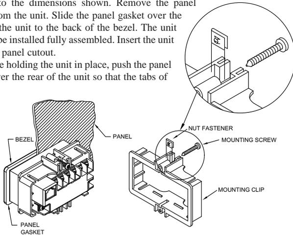
the panel latch engage in the slots on the case. The panel latch should be engaged in the farthest forward slot possible. To achieve a proper seal, tighten the latch screws evenly until the unit is snug in the panel (Torque to approx. 28 to 36 in-oz [0.202 to 0.26 N-m]). Do not over-tighten the screws.
