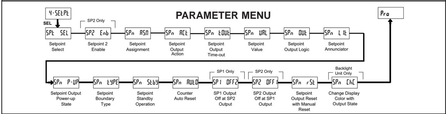
The Setpoint Output Parameters are only active when an optional Setpoint Output Module is installed in the meter. Some parameters in the menu will not appear depending on the Setpoint Assignment and Setpoint Output Action. The Setpoint Parameter Availability chart below illustrates this.
