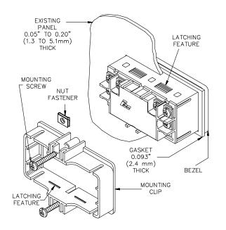
80% of its original thickness. (Recommended torque is 28 to 36 in-oz.) If not, gradually turn mounting screws to further compress gasket.
