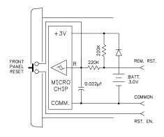
Connecting a wire from the "RST. EN." (Reset Enable) Input terminal to Common will enable the front panel Reset button.
