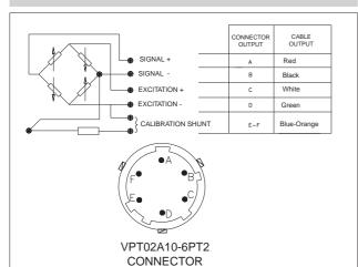
If the transducer is supplied complete with prewired connection cable, the colour code is that indicated in the table.
