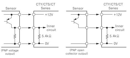
\*INPUT circuit of INA, INB, INH(INHIBIT), BATCH RESET, RESET are the same.
