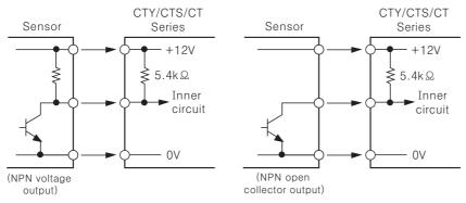
\*INPUT circuit of INA, INB, INH(INHIBIT), BATCH RESET, RESET are the same.
