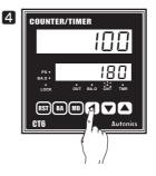
Pressing (MD) key to complete the Batch setting will return Counter to the RUN mode. (BA.S LED OFF display)
