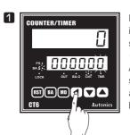
Press (BA) key in RUN mode, it will enter into the program state of Batch setting value. (BA.S LED ON display)
