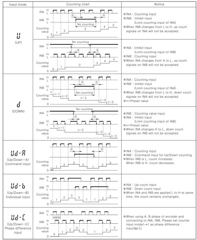
※ ♠: Over Min. signal width, ⊕: Over 1/2 of Min. signal width.
