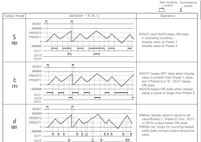
\*The output of single preset operates of double preset type.
