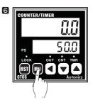
Pressing ND key to complete the setting time then return to RUN mode.
