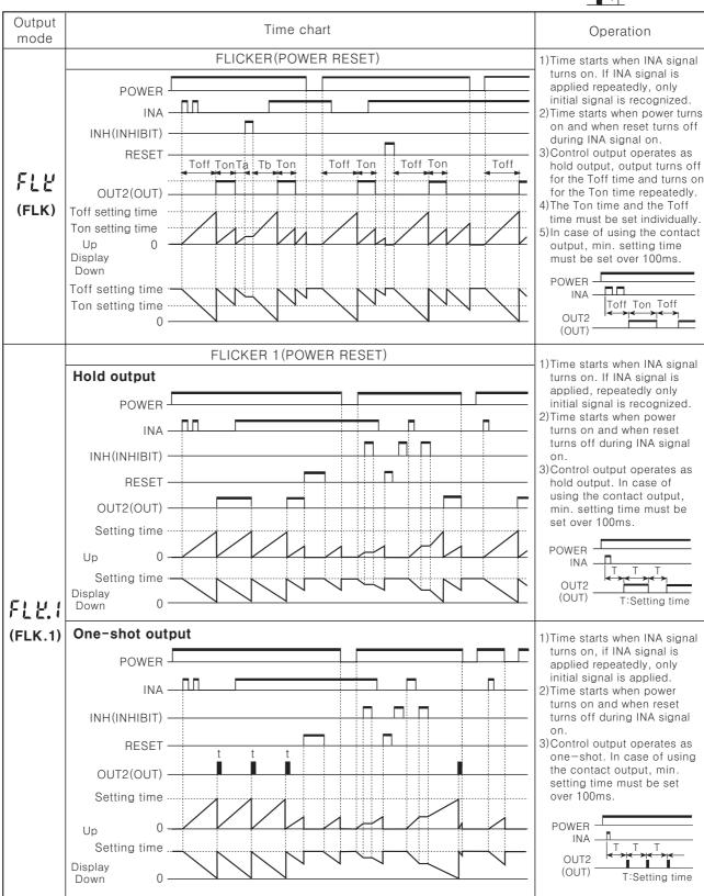
$\ensuremath{\text{\#POWER RESET}}\ : \ There \ is \ no \ memory \ retention. \ (Timer \ resets \ to \ initial \ value)$
