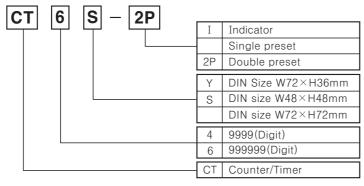
\*When using double preset type as timer mode, setting time is limited in one preset time.
