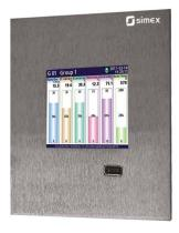
Panel mount MultiCon CMC-99SL is featured by a shallow casing — only 50 mm! All connectors are introduced on side walls of the device as in a typical panel computer. As the number of measurement inputs and outputs is limited, this design in intended mainly for systems with a small number of signals or systems which include other measurement systems with Modbus RTU interface. An Ethernet interface is also available to upgrade every MultiCon control's application easily.
