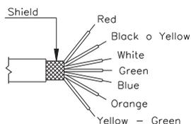
\* The screen is isolated from the transducer body. It is recommended that the ground is connected at the instrument end.
