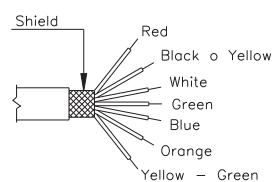
\* The screen is isolated from the transducer body.
