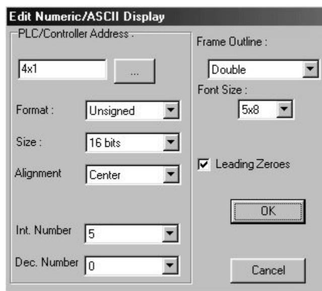
3. Enter the data as shown above (for more details on using the Numeric/ASCII Display object, consult *Chapter 8: Entering and Displaying Numeric and ASCII Characters*.)
