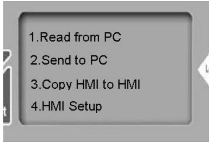
9. Press the **F1** key to move the block cursor to 1. *Read from PC*, and then press the ENTER key on the BLU300. The BLU300 will display a screen indicating that it is waiting for communications to be established with the BlueLeaf software.
