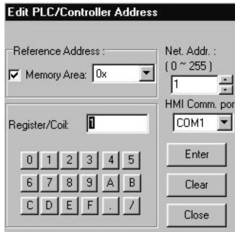
4. Check the **Memory Area** box. Click the pull-down box to select the *target PLC memory area*. Use the numeric keypad to enter the specific *PLC memory address*. Select the *PLC Network Address* (if applicable) and *HMI communications port*. Click **Enter** to go back to prior dialog box.
