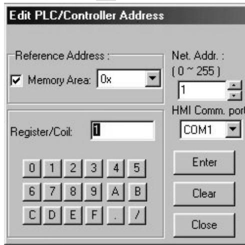
8. Check the **Memory Area** box. Click the pull-down box to select the *target PLC memory area*. Use the numeric keypad to enter the specific *PLC memory address*. Select the *PLC Network Address* (if applicable) and *HMI communications port*. Click **Enter** to go back to prior dialog box.
