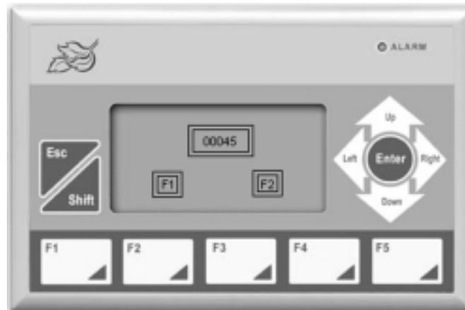
7. Press the **F1** key to increment the value in the Numeric Display object. Press the **F2** key to decrement the value in the Numeric Display object.
