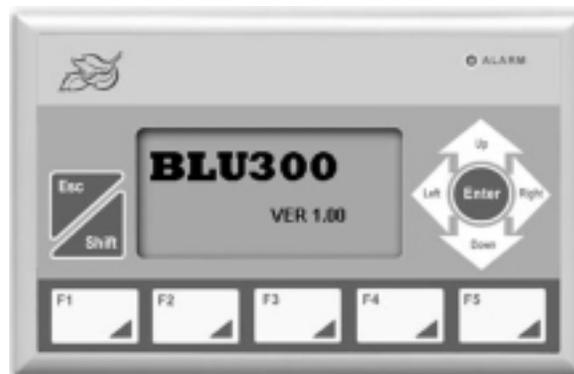
When enabled, this screen briefly appears whenever the OIT is powered up. Then the first screen of your project is displayed.
