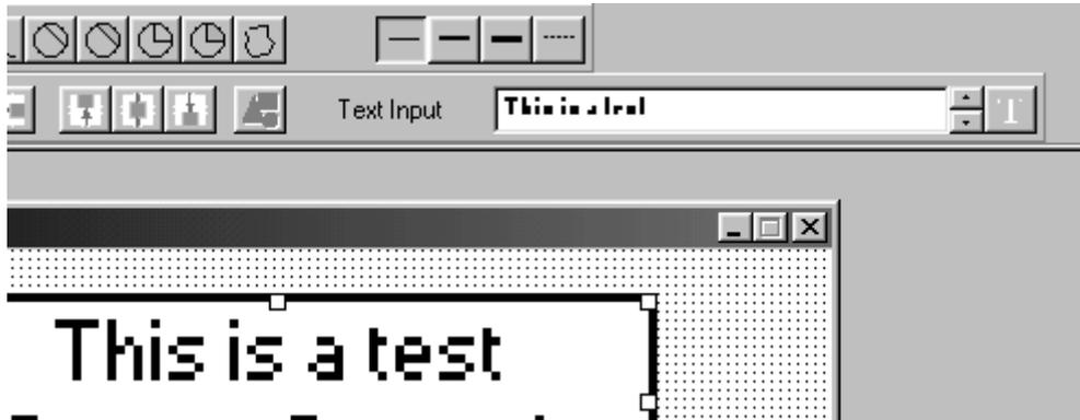
1. You can edit the text of a text box by clicking on the text object and then making changes in the Text Input box located on the Text/Graphic Toolbar.
