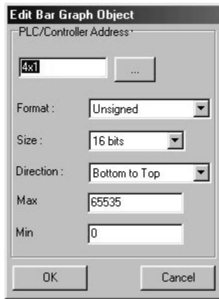
2. In the **PLC/Controller Address** frame, enter the *PLC coil or controller address*. Or click the PLC/Controller Address button to display the Edit PLC/Controller Address dialog box:
