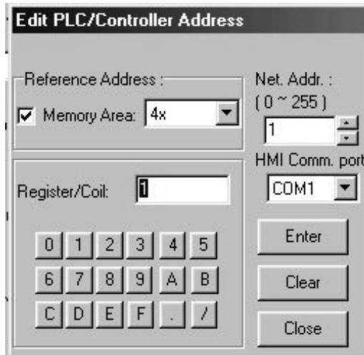
15. Check the **Memory Area** box. Click the pull-down box to select the *target PLC memory area*. Use the
