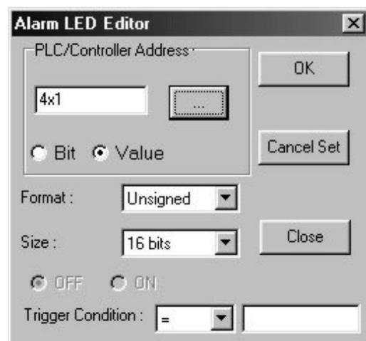
2. First select either **Bit** or **Value** to determine if the Alarm LED will read from a PLC coil or a PLC register (16 or 32 bit).
