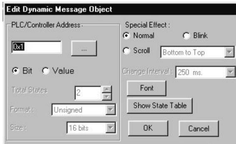
2. Check **Bit** to select a PLC coil. Check **Value** to select a PLC register.
