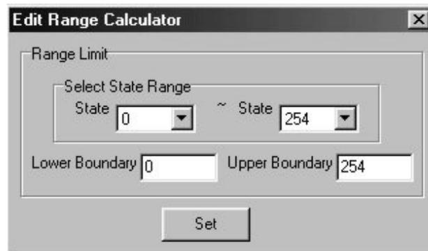
The Range Calculator is a tool to help you easily determine the ranges. By setting the minimum value to be represented (lower boundary) and maximum value to be represented (upper boundary), the calculator will evenly divide the range for each state. Click the **Set** button to go back to the prior dialog box.
