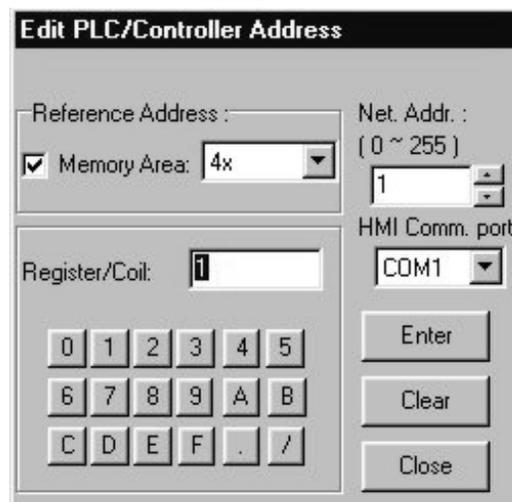
3. Check the Memory Area box. Click the pull-down box to select the *target PLC memory area*. Use the numeric keypad to enter the specific *PLC memory address*. Select the *PLC Network Address* (if applicable) and *HMI communications port*. Click **Enter** to go back to prior dialog box.
