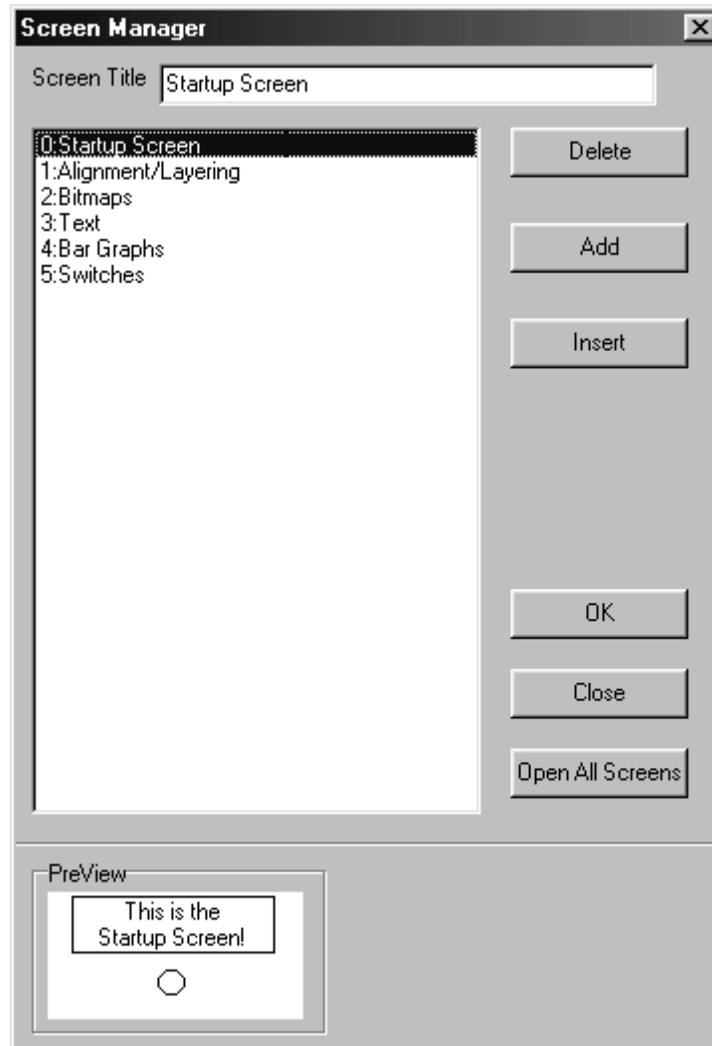
2. The Screen Manager allows quick screen selection for editing. You can also create a new screen, delete an existing one, or insert a new screen between pre-existing screens. To view all of the screens of the project, click the **Open All Screens** button. The Preview area provides a quick preview of the screen being selected.
