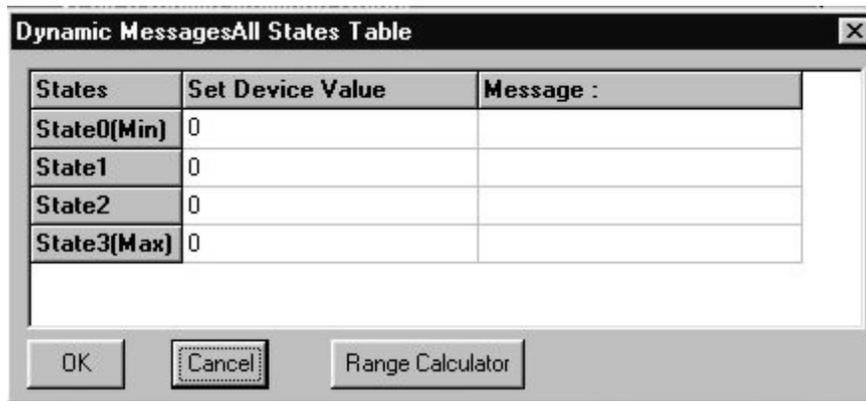
12. For each State, enter the *Range Limit* that determines if that state's text message is to be displayed. The range limit number entered must be larger than the prior state and smaller than each successive state, as shown in the example above. You can also click the **Range Calculator** button to display the Range Calculator:
