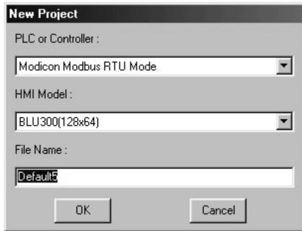
2. Select the *PLC or controller* that you are using from the **PLC or Controller** pull-down box.
