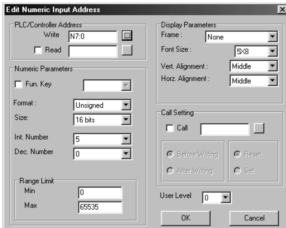
2. In the **PLC/Controller Address** frame, enter the *PLC* or *controller address* you wish to access in the
