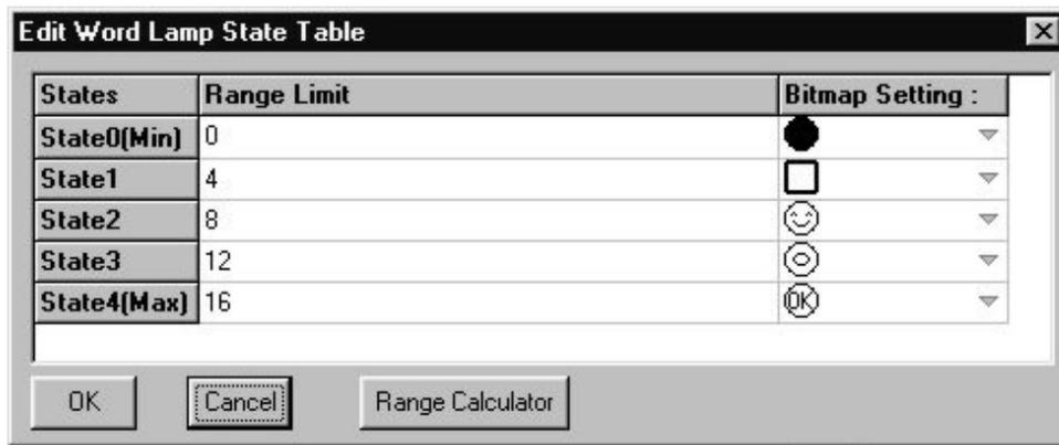
7. For each State, enter the *Range Limit* that determines if that state's bitmap is to be displayed. The range limit number entered must be larger than the prior state and smaller than each successive state, as shown in the example above. You can also click the **Range Calculator** button to display the Range Calculator:
