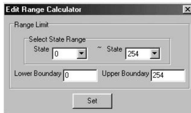
13. The Range Calculator is a tool to help you easily determine the ranges. By setting the *minimum value* to be represented (lower boundary) and *maximum value* to be represented (upper boundary), the calculator will evenly divide the range for each state. Click the **Set** button to go back to the prior dialog box.
