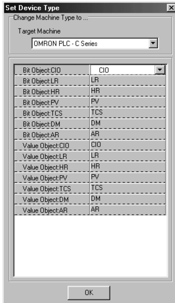
2. Use the Target Machine dialog box to select which PLC you want to use. The window will show a list of supported registers for the PLC chosen.
