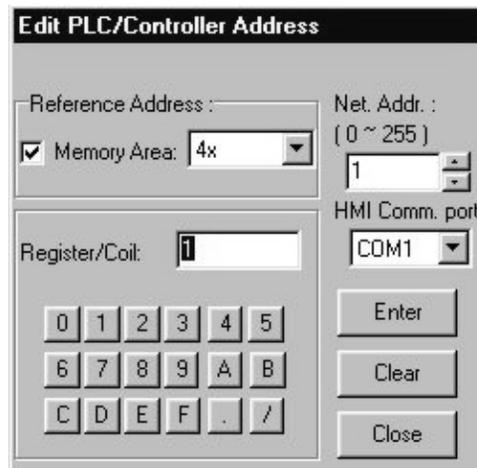
Check the **Memory Area** box. Click the pull-down box to select the *target PLC memory area*. Use the numeric keypad to enter the specific *PLC memory address*. Select the *PLC Network Address* (if applicable) and *HMI communications port*. Click **Enter** to go back to prior dialog box.
