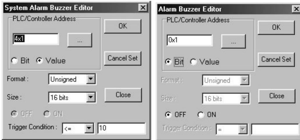
2. First select either **Bit** or **Value** to determine if the Alarm Buzzer will read from a PLC coil or a PLC register (16 or 32 bit).
