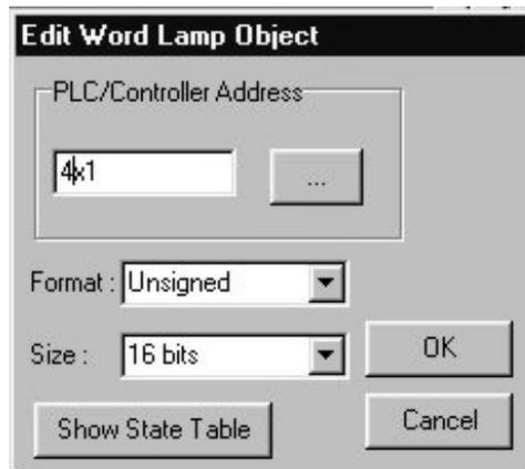
2. In the **PLC/Controller Address** frame, enter the *PLC coil* or *controller address*. Or click the PLC/Controller Address button
