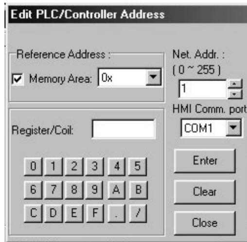
16. Select either **Before Writing** or **After Writing**. This determines whether the coil is written to before the new value is written to the PLC register or immediately after when the Enter key is pressed. Select either **Reset(0)** or **Set(1)** to determine which value is written to the PLC coil.
