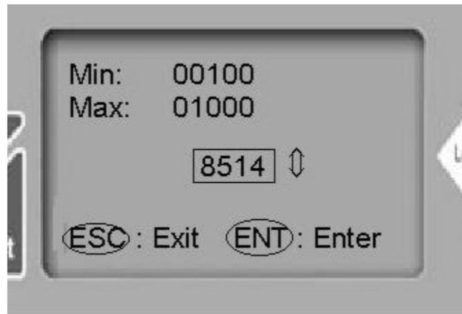
13. The Numeric Entry screen displays the minimum and maximum allowed values at the top of the screen (in this example- Min:100 Max:1000). In the center of the screen, the current value of the PLC register is displayed (note: if you checked the Read checkbox during configuration of the Numeric Input object, then the HMI will show the latest value of the Read register).
