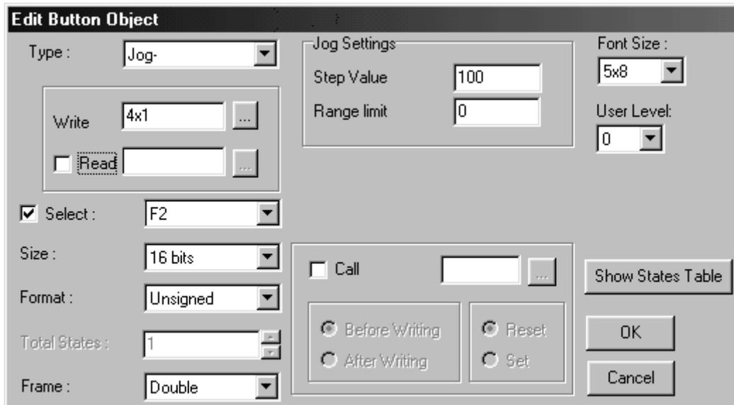
6. Enter the data as shown above (for more details on using the Function Key object, consult *Chapter 9: Using the Function Keys* )
