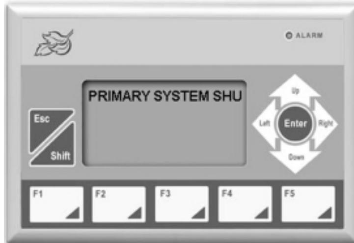
To remove the alarm, enter value 11. This will blank the OIT screen, turn off the buzzer and LED.
