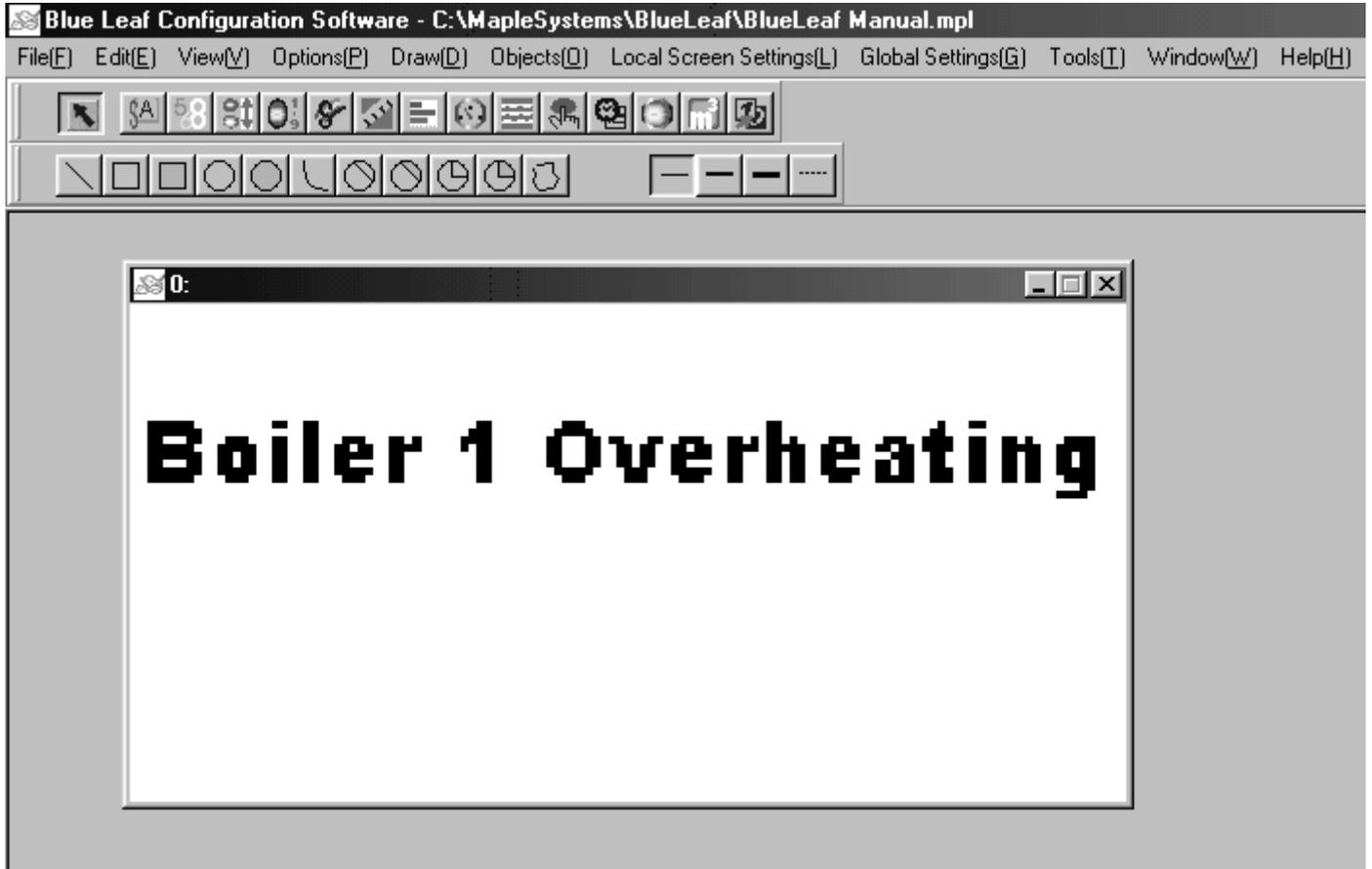
Now download your project to the BLU300 Series OIT. Enter the value 1 into the PLC register you are using for the alarm (in this example, 4x1). The following should be displayed on the OIT, with the Alarm LED on and the buzzer pulsing:
