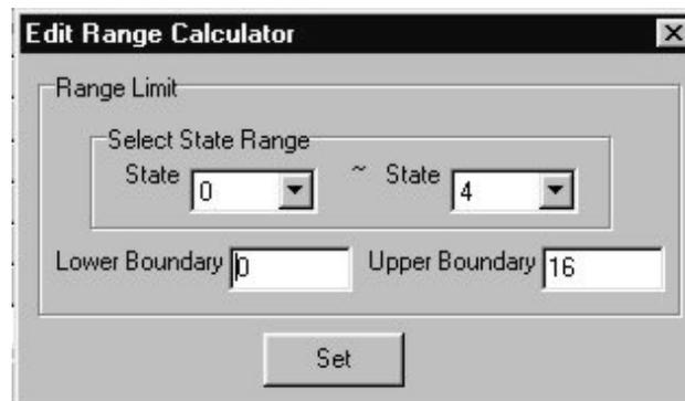
8. The Range Calculator is a tool to help you easily determine the ranges. By setting the minimum value to be represented (lower boundary) and maximum value to be represented (upper boundary), the calculator will evenly divide the range for each state. Click the **Set** button to go back to the prior dialog box.
