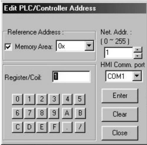
The **Edit PLC/Controller Address** dialog box contains the following fields and controls:
