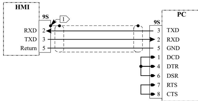
**OIT to PC Serial Port Pin Assignments**
