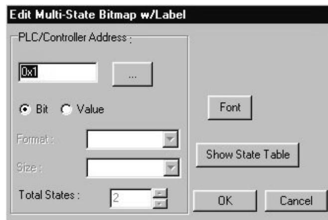
2. First select either **Bit** or **Value** to determine if the Multi-State Bitmap object will read from a PLC coil or a PLC register (16 or 32 bit).
