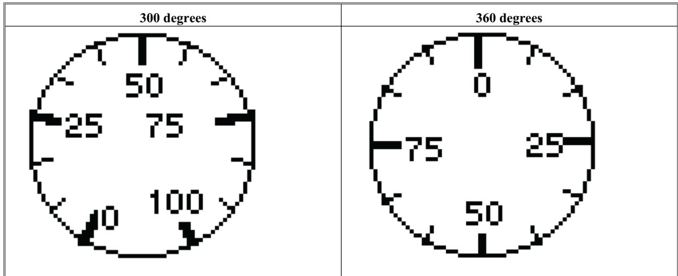
Data in the PLC register can be interpreted as unsigned, signed, BCD, or hexadecimal. You can select the minimum and maximum range displayed, then select the number of major delineations (tick marks) as well as minor delineations (minor tick marks).
