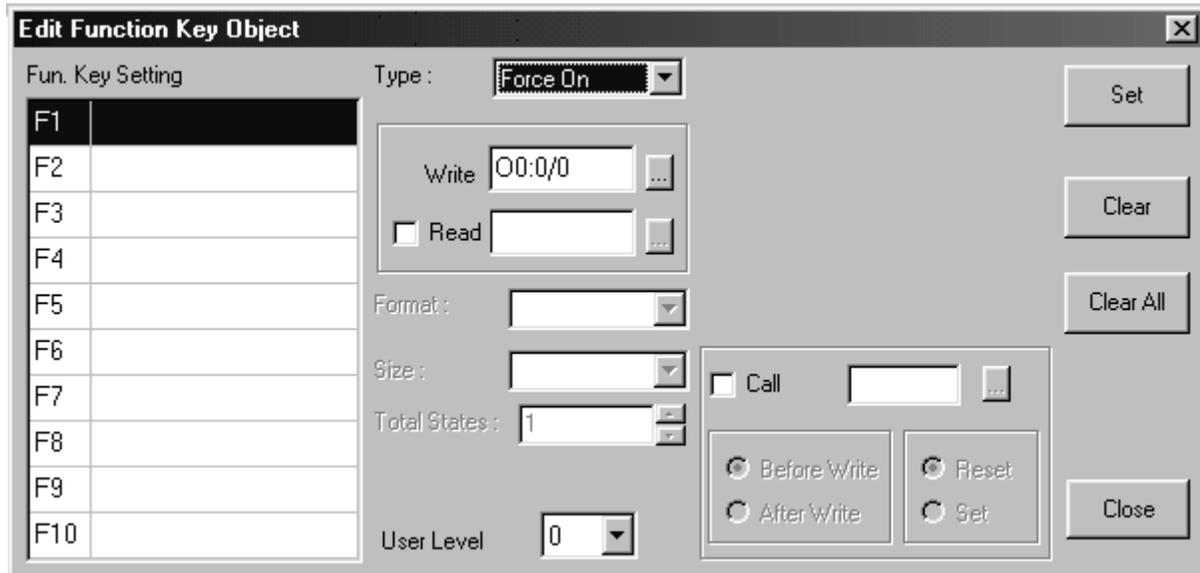
2. Click on the *function key* (F1 thru F10) that you wish to configure. Note: F6-F10 correspond to shift F1-F5 keys. Configure the parameters for the function key per type used. When finished, click the **Set** button, then define the next function key or click the **Close** button. Use the **Clear** button to clear a particular function key or the **Clear All** button to erase settings for all function keys.
