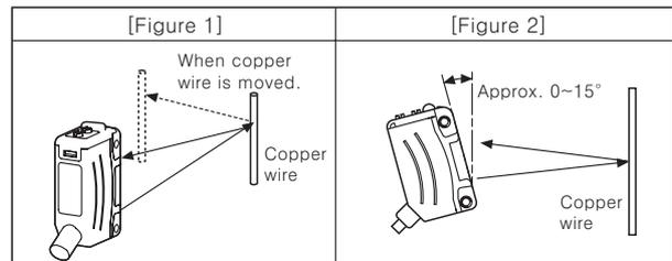
※ Mount sensor slanted at an angle ranged 0~15° shown above as [Figure 2] for stable detection to detect as shown in [Figure 1].
