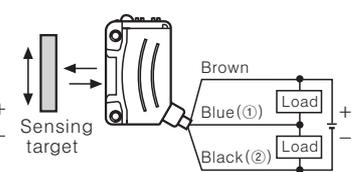
※ ① : The load connection of NPN open collector output, ② : The load connection of PNP open collector output
