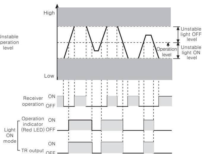
※ The waveform of 'Operation mode indicator' and 'TR output' is for Light ON mode, it is operated as reverse in Dark ON mode.
