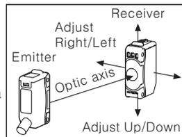
※ When the sensing target is translucent or small (Under  $\phi$  16mm), it can be missed by the sensor because the light can penetrate it.
