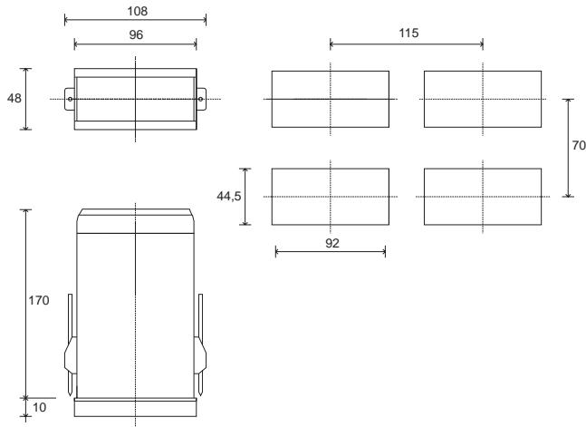
Dimensions: 96x48mm (1/8 DIN), depth 167mm
